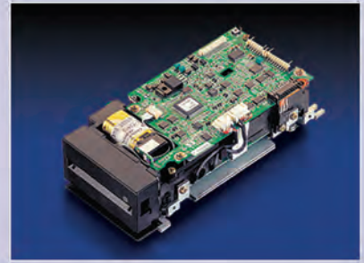
Motorised Hybrid Card Reader ICM330. Smart and Magnetic Card Reader, 1 SAM socket on board. Anti-Intrusion shutter. EMV Approval. RS232 or USB interface.
